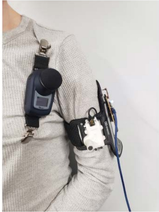
Figure 14: Mounting location of the dBadge, which has been moved closer to the ear compared to Experiment 1.
