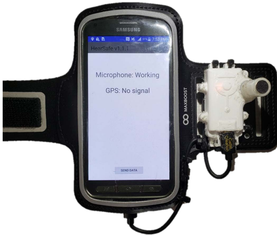
Figure 1: The HearSafe sensor which includes a water resistant arm band, custom smartphone application, noise dosimeter, and On-The-Go cable.
